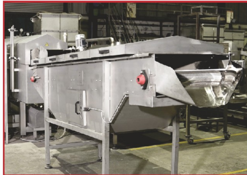
Ambient Air After-Cooler
