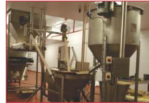
Flexible Screw Conveyor for Meal Distribution for Snack Extruder
