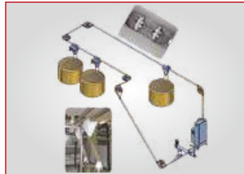
Bulk Conveying using Drag (Chain/Rope-Disc) Conveyor for Process
